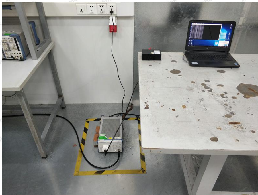
Photo of Power Line Conducted Emission Test
