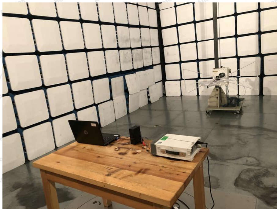
Photo of Radiated Emission Test
