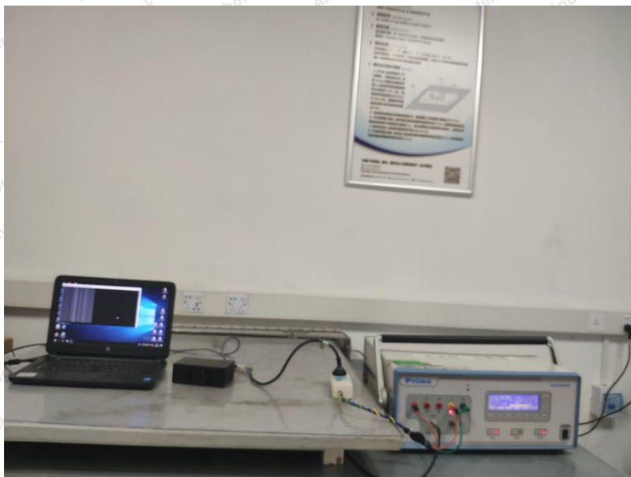
Photo of Electrical Fast Transient/Burst Immunity Test
